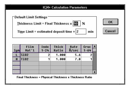
The grid in this screen displays index symbols previously defined in the Film Indices editor. Since Film Material names are read from the IC/4+ the instrument must be on when the dialog box is activated. Your entries under Film Material will match those currently programmed in your instrument. The STC-200/SQ does not store material names and you must edit the entries.
