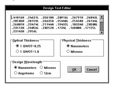
A design containing parentheses, *i.e.* (.25H .25L)10 .25H, is 'exploded' into individual layers upon returning to the Layers Editor with  $\mathbf{OK}$ . Note that this dialog box includes optical and thickness convention choices. Usually there is no need to alter these settings since they are loaded with the design.
