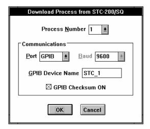
This screen also appears after clicking **Upload <Ctrl+U>** and can be accessed via **File...Communications...Port**. Note that **GPIB Checksum ON** applies only to the Sycon STC-200/SQ and is otherwise dimmed.
