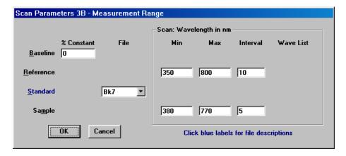
The above dialog can be accessed directly from the Main Menu by clicking **Setup...Measurement Range <Ctrl+A>**. Press OK or Cancel once more for the final Scan Method screen - Graph Axes.
