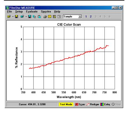
We start by examining the Scan Method (see "Instrument Settings" on page 19) which are edited in linked dialog boxes. Click **Setup...Scan Method <Ctrl+M>**. a Scan Method includes instrument settings, graph ranges, etc. As shown below, Screen 1A selects the *Input Device* which can be a spectrophotometer, digitizer (rarely utilized), or server (raw or processed data).
