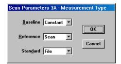
We plan to measure the reflectance of AR coatings on BK7 substrates over the CIE color range 380-780 nm. Since previous experience indicates that best accuracy is obtained if we scan an uncoated substrate (ground second surface) at the start of each measurement series, we enter *Scan* next to *Reference*.
