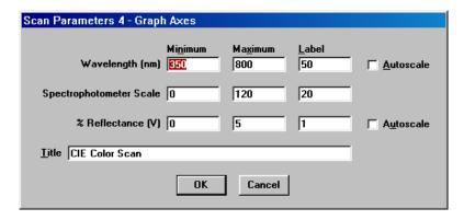
Range and Axes can be edited by without looping through the entire Scan Method. This dialog can be accessed from the Main Menu by clicking **Setup...Graph Axes <Ctrl+G>**. Note that MEASURE displays different graphs during and after the scan. While scanning the graph monitors actual values sent by the spectrophotometer. Here the vertical scale is set by **Spectrophotometer Scale** settings. This scale is also used for Baseline and Reference readings.
