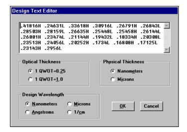
A design containing parentheses, *i.e.* (.125H .25L .125H)10, is 'exploded' into individual layers upon returning to the Layers Editor. Adjacent layers of the same type are combined when there are parentheses. That is .125H .125H becomes .25H. (Adjacent layers are NOT combined in the Layers Editor. This makes it possible to break up thick layers into thinner layers of the same type.)
