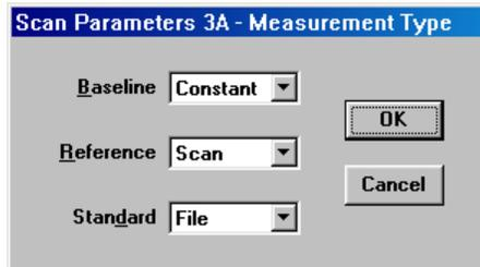
We plan to measure the reflectance of AR coatings on BK7 substrates over the CIE color range 380-780 nm. Since previous experience indicates that best accuracy is obtained if we scan an uncoated substrate (ground second surface) at the start of each measurement series, we enter *Scan* next to **Reference**.
