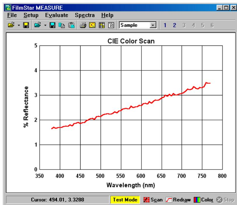
We start by examining the Scan Method (see “Instrument Settings” on page 19) which are edited in linked dialog boxes. Click **Setup...Scan Method <Ctrl+M>**. a Scan Method includes instrument settings, graph ranges, etc. As shown below, Screen 1A selects the **Input Device** which can be a spectrophotometer, digitizer (rarely utilized), or server (raw or processed data).
